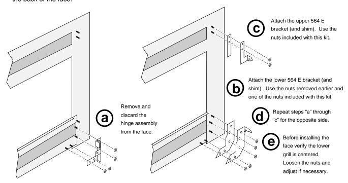
3 Pull the electric fireplace out of the mantel (or built-in location). Attach the cove covers and face following the directions below. Slide the fireplace back into place to complete the installation.
